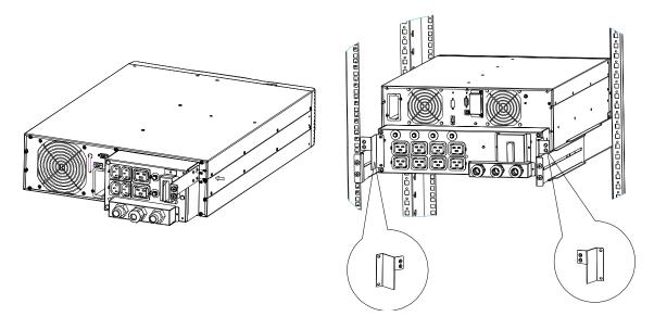
Figure 3-12. Install the PDU's ears to the UPS
