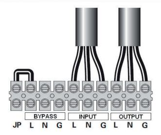
Figure 4-2. Common input sources connection
