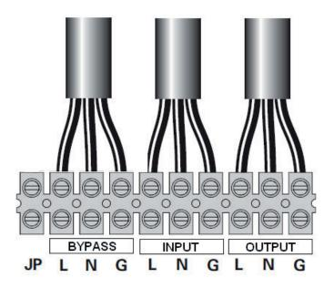
Figure 4-3. Separate input sources connection
