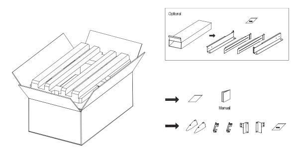
Figure 3-2: Unpacking the carton of 10K UPS
