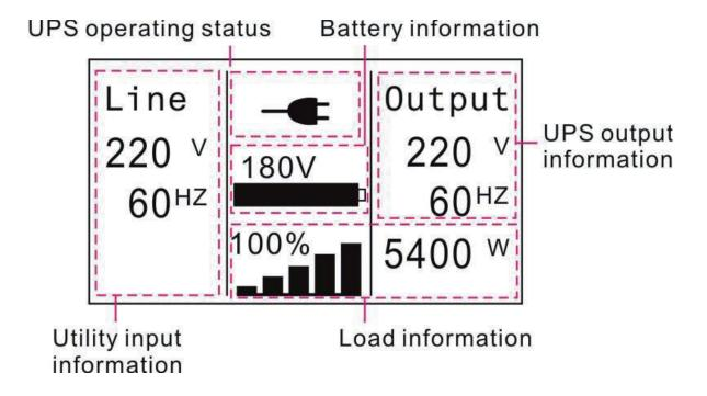
Figure 5-2 The default LCD display
