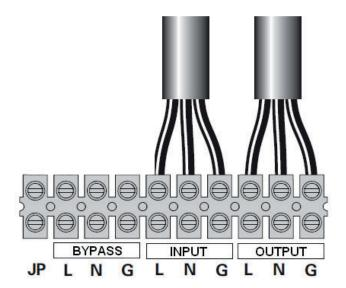
Figure 4-4. Frequency converter connection
