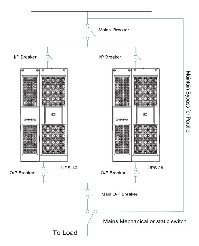
Figure 4-5.b: Parallel System Installation Diagram
