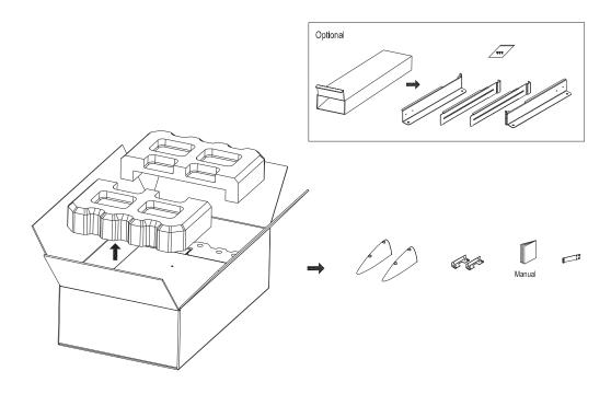
Figure 3-1: Unpacking the carton of 6K UPS
