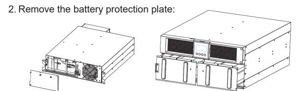
Figure 3-9. Removing the Battery Protection Plate
