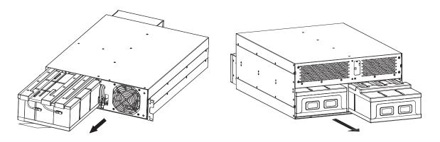
Figure 3-11: Removing the Battery Tray
