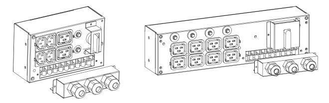
Figure 4-1. PDU of 6K/10K
